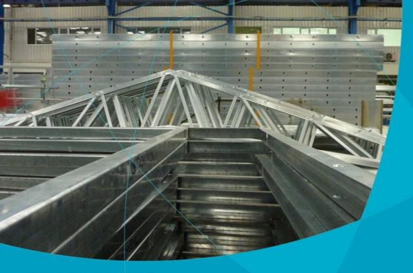
The roof trusses and mezzanine floor coverings of Nestavilla, that are connected with bolts without the need for welding, are producing in American origined production lines.
